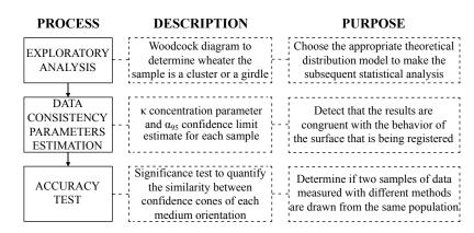
Figure 2. Flow chart for the implementation of the three tests conforming the methodology proposed in this work.
