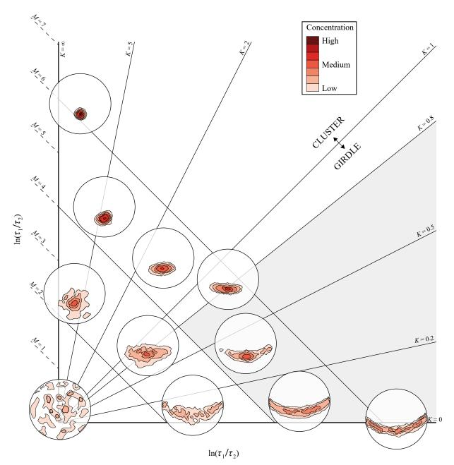
Figure 3. Woodcock's diagram showing the cluster's (circularly symmetric) and gridle's (axially symmetric) fields. (Modified from Woodcock, 1997). Observe that the definition of Cluster or Girdle depends on the coordinate of the data points with respect to line K=1. Where  $K = ln(\tau_1/\tau_2)/ln(\tau_2/\tau_3)$ , and  $M = ln(\tau_1/\tau_3)$ .
