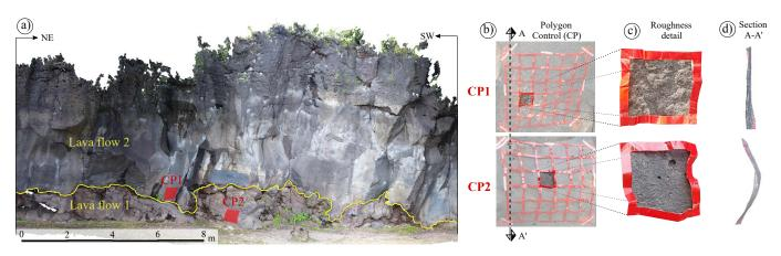
Figure 4. "La Escuelita" rock outcrop wall (19.3341°, -99.1933°). (a) Panoramic view, yellow polyline indicates a discontinuity surface between two lava flows and red polygons show the location Control Polygons 1 and 2. (b) Red meshes show the discretization, of CP1 corresponds to a planar discontinuity surface, while CP2 corresponds to a curved one. (c) Roughness detail for one element on the mesh. (d) Show a section of planar surface (CP1) and curved surface (CP2).
