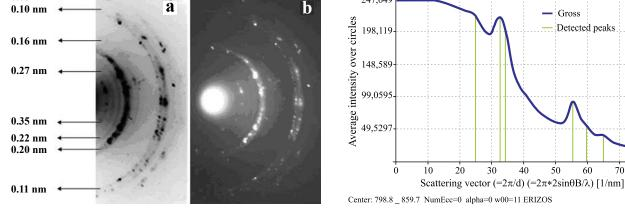
Figure 6. a, b:Selected area electron diffraction (SAED) pattern from many thorns as those shown in Figure 4; (a) shows the inverse contrast from (b) for clarity. This polycrystalline diffraction pattern can be indexed as K<sub>3</sub>(VS<sub>4</sub>) and as cristobalite. C: SAED intensities profile obtained from process diffraction software package (one region of the sample with the "hedgehog"-like particles).
