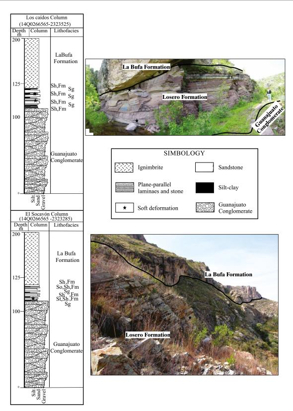
Figure 3. Lithostratigraphic columnar section of the Los Caídos and El Socavón localities. Facies, Fm: mudstone with desiccation cracks; Sg: coarse sandstone of brown color with normal gradation; Sh: medium to fine sandstone with plane parallel laminae and associated desiccation cracks; So: medium to fine sandstone with ripples of green color; St: medium sandstone with antidunes and cross laminations of green color.
