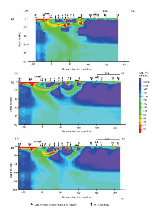
Figure 6. Resistivity models for profile MT-1 using the same parameters for inversion. a: Soundings rotated to the regional strike (N9W) and projected along a profile perpendicular to the MT transect; b: the inverted polarity model; and c: rotated to the principal axis (Swift, 1967) model. Generally speaking, the three resistivity images show the same enhanced conductivity zones and resistive features. TZR: Tepic-Zacoalco rift; AR: Ameca river.
